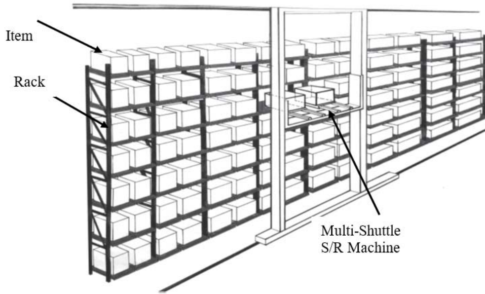
FIGURE 1. A TWIN-SHUTTLE AUTOMATED STORAGE/RETRIEVAL SYSTEM (YANG, PENG, YE, AND MIAO, 2017)
